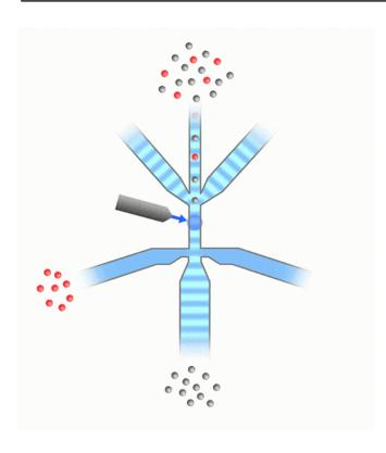
On-chip Sort uses a small disposable microfluidic chip (with either 80  $\mu$ m or 150  $\mu$ m flow channel width) as the core of its technology. Sample and sheath fluid are loaded into the sample and sheath reservoirs on the chip, respectively. Unlike conventional cell sorters, that require a specific sheath fluid, On-chip Sort allows for the use of any sheath fluid appropriate for your cells (e.g., culture medium, fresh water, sea water, oil).
